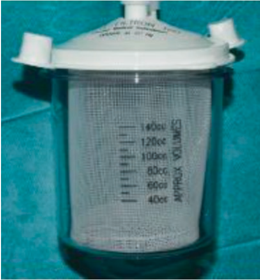
Fig. 6.9 Detailed view of the filter unit with pores 800 \mu\text{m} in diameter
