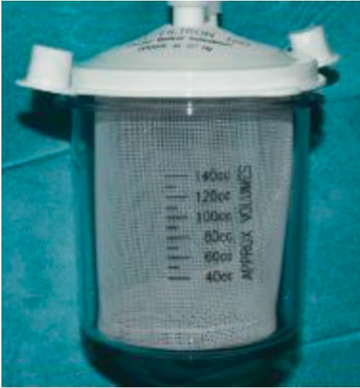
Fig. 6.9 Detailed view of the filter unit with pores 800 \mu\text{m} in diameter
