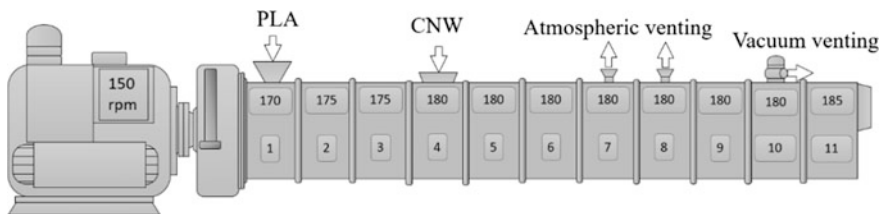
Fig. 2 Schematic image of extrusion process with liquid feeding [26]
