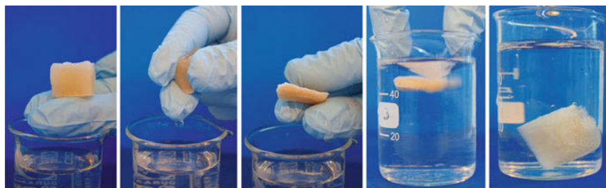
Fig. 29 The repeatable liquid water absorption capacity of the aerogels that maintained their structure and shape in water (Reproduced from [172] with permission)
