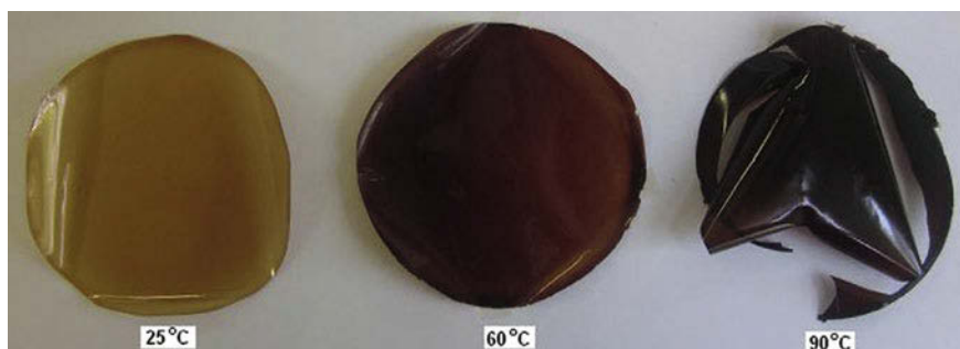
Fig. 21 Films obtained from hemicelluloses isolated at the end of pretreatments conducted at 25, 60 and 90 \text{ }^\circ\text{C} (Reproduced from [134] with permission)
