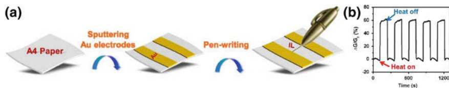
Fig. 2 a Fabrication process showing ionic liquid (IL) paper chip written with a pen, b thermal response with on-off cycles of the paper chip between 45 and 25 °C. Adapted with permission from Ref. [27] © 2017 ACS publisher
