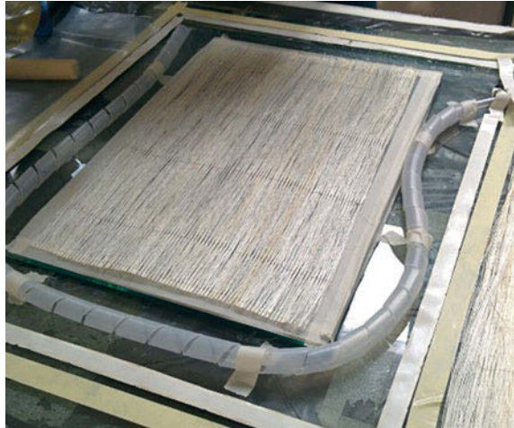
Fig. 10 a unidirectional ‘stitched’ fabric of agave fibre obtained in laboratory
