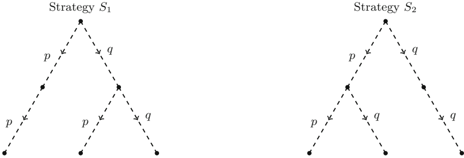
Fig. 2. Two strategies S_1 and S_2 for n = 3 . The cost of S_1 is 3p + 2q , and the cost of S_2 is 2p + 3q . S_1 is optimal when q \geq p and the number of processors is K = 1 . Isogeny computations in S_1 cannot be parallelized. The parallelized cost of S_2 is 2p + 2q . Therefore, S_2 is optimal for all p, q when K = 2 , even though it is not optimal when K = 1 and q > p .
