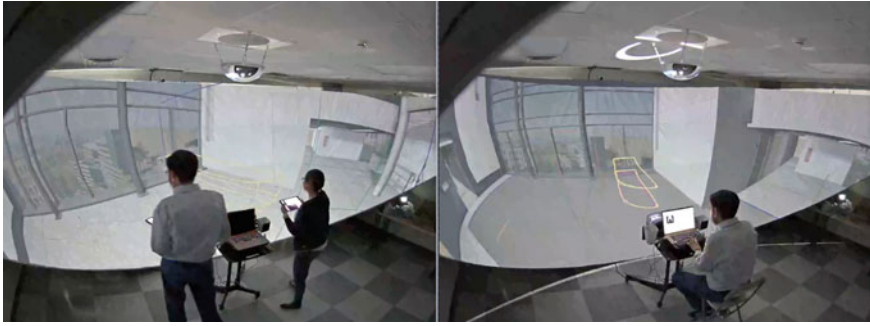
Fig. 1 Immersive co-design sketching system (Hyve-3D) used during the co-design sessions (left) and the immersive self-observations experience assessment (right)
