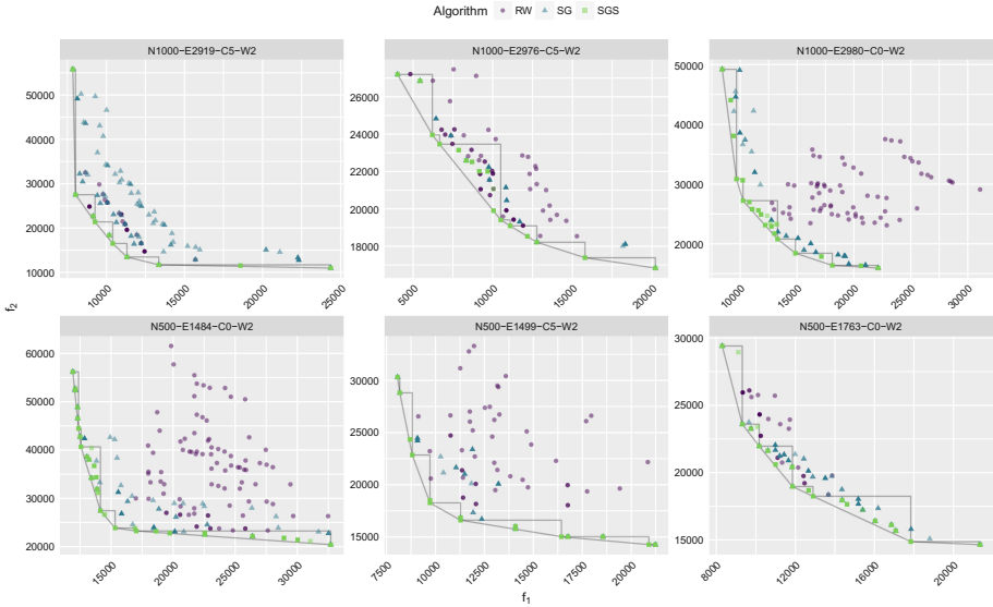
Fig. 5. Union of Pareto-front approximations of each 10 runs of all algorithms on some instances with n = 500 and n = 1000 nodes respectively. The instance names are encoded as follows: N<#nodes>-E<#edges>-C<#clusters>-W<#weights> where 0 clusters indicates unclustered, i. e., random, instances.
