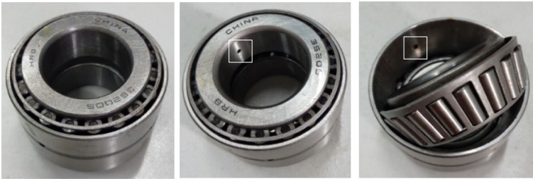
Fig. 2. Figures of experiment bearings: (a) normal; (b) inner race fault; (c) outer race fault
