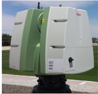
Terrestrial laser scanning
