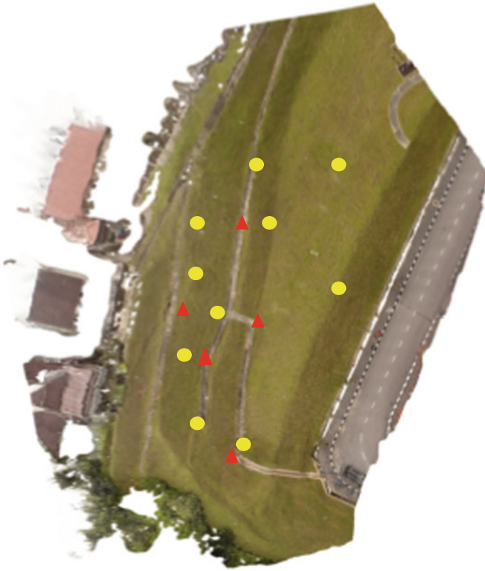
Fig. 9 Distribution of GCPs and CPs of the slope area
