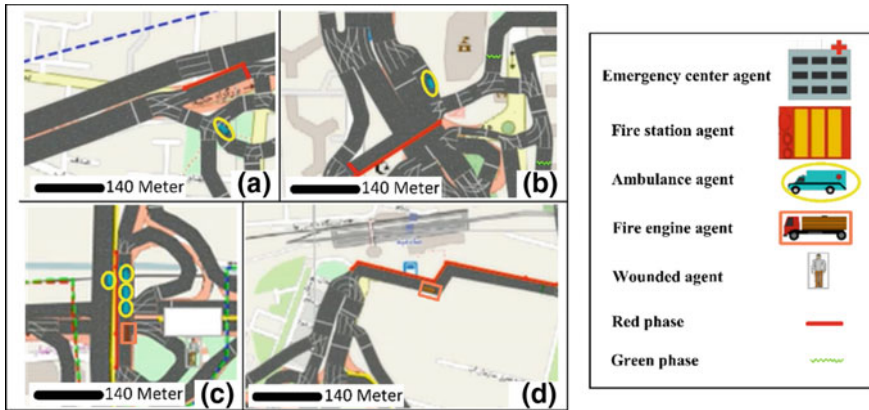
Fig. 13 The actions of the ambulance and fire engine agents. a and b Updating of the ambulance route when faced with the blocked street in the second and third type of the multi-agent rescue operation model, c Resolving the blocked street by the fire engine in the first type of the multi-agent rescue operation model, d Resolving the blocked street by the fire engine in the second and third types of the multi-agent rescue operation models
