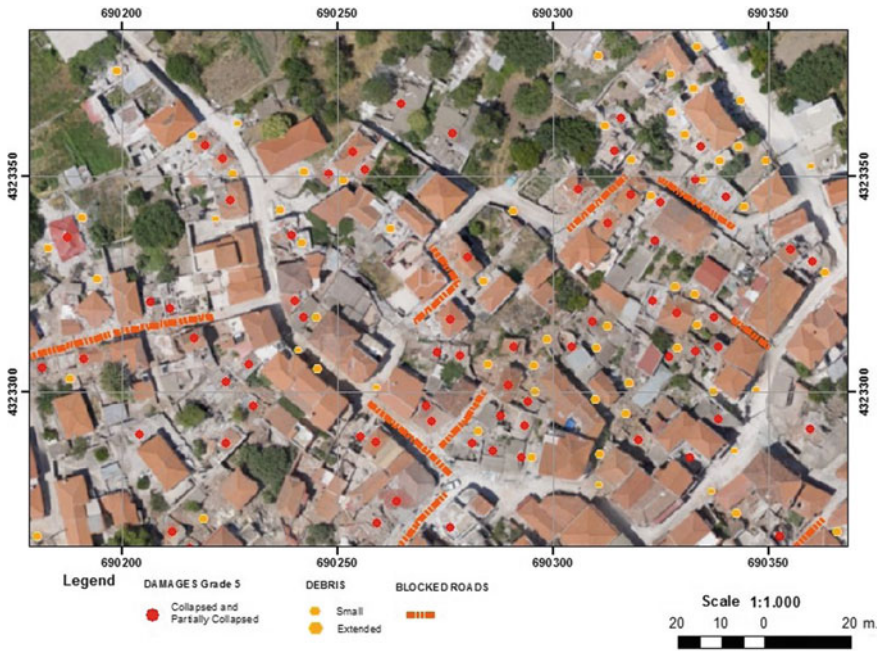
Fig. 8 Orthophoto map of 13th June 2017 at a scale of 1:1.000 showing the NW part of Vrisa settlement which concentrates a large number of building of grade damages 5 e.g. partial and total collapse of buildings, the blocked roads and the areas with debris
