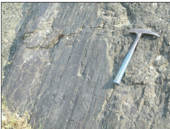
Fig. 3 Characteristic example of a slickenside in the broader area (successive stages of brittle, semi-brittle & ductile deformation are evident throughout the ophiolitic mass)
