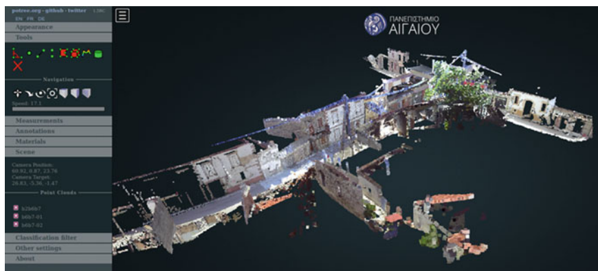
Fig. 5 Web-application (Potree) of the “Vrisa project” showing three interconnected 3D-scans in the main square of the village
