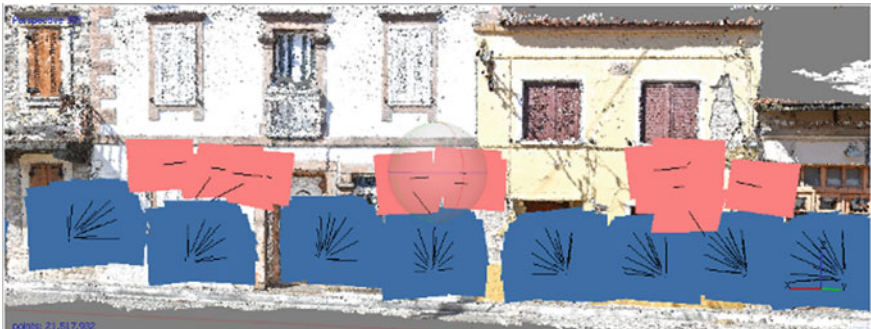
Fig. 5 Projection centers at street level (blue) and by using mounting pole (pink)
