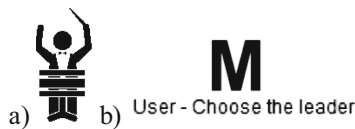
Fig. 4. (a) Symbol of the root node of a model describing how a set of task models is orchestrated, and (b) Representation of an entire task model that is used inside an orchestration model
