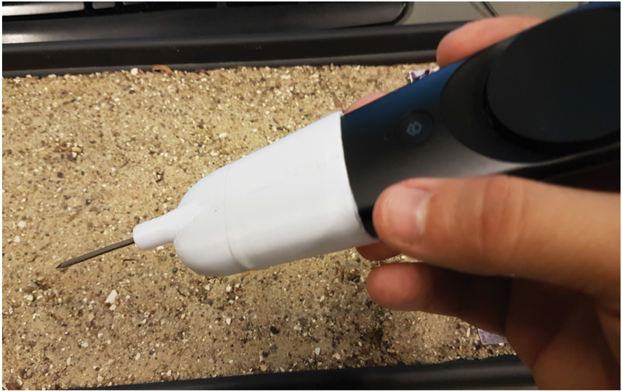
Fig. 7. The needle used for the experiment, made from a 3D printed mount and a nail and attached with a bolt in the loop designed for the wrist strap.
