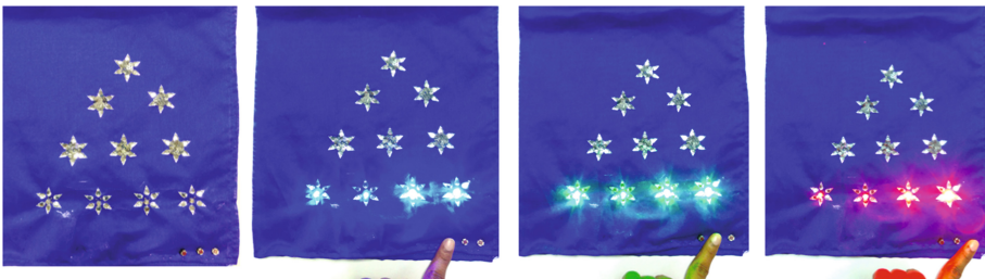
Fig. 6. Aster – Static and Dynamic - three colors controlled by three buttons (Color figure online)
