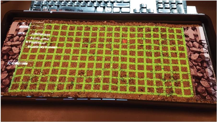
Fig. 5. The grid projected onto the sand with the targets shown as a red dot. (Color figure online)
