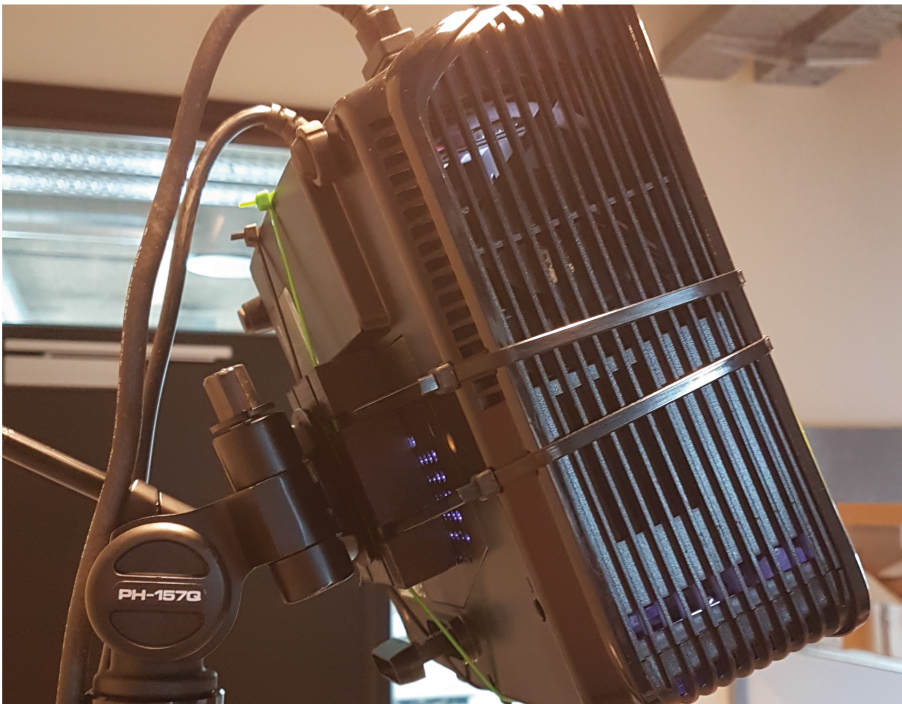
Fig. 4. The projector mounted for the top-down projection setup.
