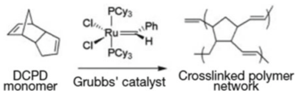
Fig. 2.1 Polymerization of DCPD activated by Grubbs' catalyst. Reprinted with permission from White et al. (2001)
