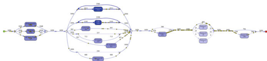
Fig. 8 The process model discovered from the sepsis event log by the Inductive Visual Miner (filtered to show 80% of paths). Alignment information is overlaid on the model. More frequent paths and activities are colored darker
