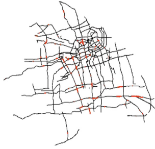
Fig. 5. Spatial distribution of congested road segments in road network.
