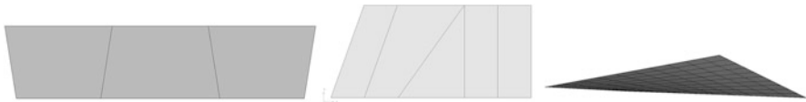
Fig. 5.6 Quadrilateral elements with mesh quality exceed the minimal in-house recommended values of a Jacobian of 0.7 (left); internal angle of 55 degrees, 10 degrees exceeding the recommended 45 degrees (centre); and a warpage of 1.65 (right)
