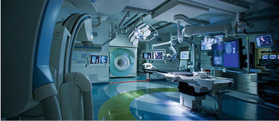
Fig. 12.5 A view through the AMIGO Suite's advanced operating room into the adjoining MR imaging room. The doors to the adjoining room are closed during most of the procedure so that standard equipment can be used for surgery. When the surgeon needs an updated image of residual tumour, non-magnet safe equipment are removed from the operating room, the doors are opened, and the magnet is moved into the operating room on ceiling mounted rails. After imaging, this process is reversed and surgery can resume. Moving the equipment and the magnet adds significant time to the surgical procedure, so iMRI is typically only performed once per surgery
