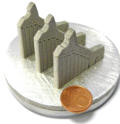
Fig. 1. Tensile test specimens, made from AZ31 with SLM technology.
