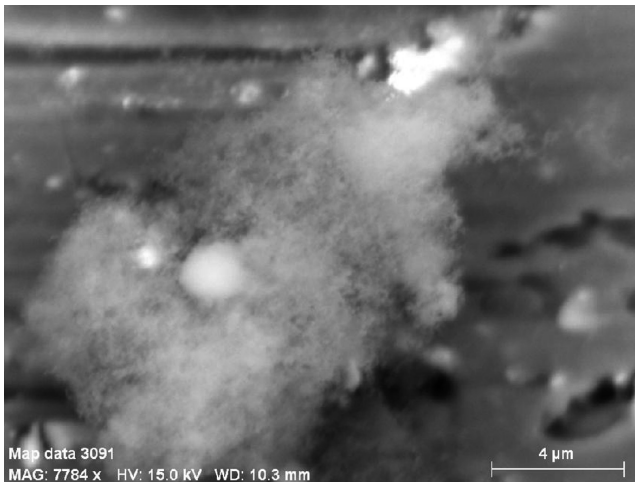
Fig. 5. Cauliflower like products of magnesium evaporation.
