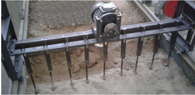
Fig. 8. Industrial platform with feed elements is installed in the vibroscreen trough, built on the data basis of finite element modeling and analysis
