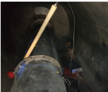
Fig. 7. Measurement system: a) impact hammer, sensors, and data recorder, b) the spectrum of the system's response to vibrations forced in the vertical direction
