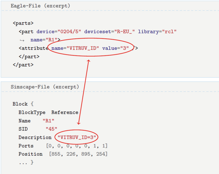
Fig. 2. Annotation of identifiers through adding attributes to the Eagle file and block comments to the Simscape file
