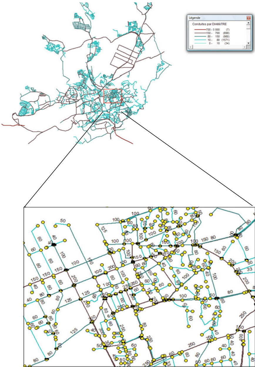
Fig. 7.9 Thematic analysis of Tlemcen urban cluster's network according to distribution of diameters
