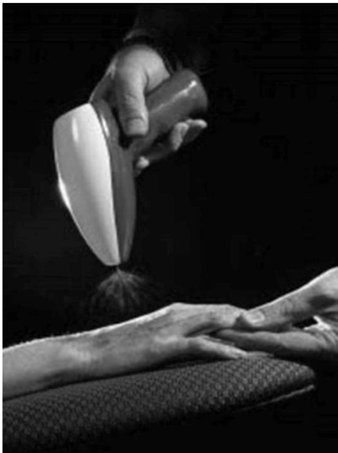
Fig. 22 Handy ES machine generating NFs for dressing the wound (Huang et al. 2003) Copyright 2003. Reproduced with permission from Elsevier Ltd.
