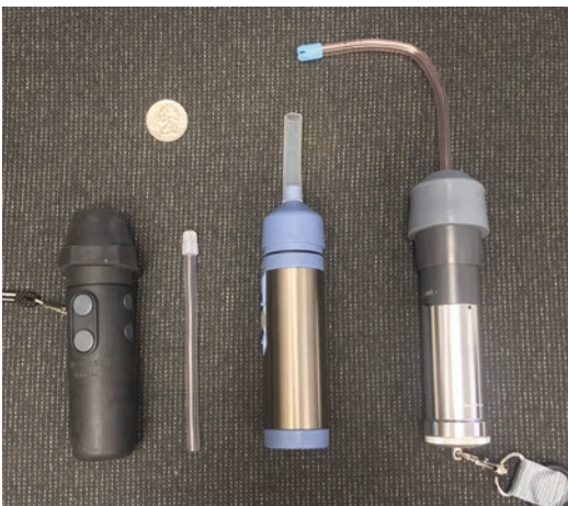
Fig. 9.3 Neck-type electrolarynges, with quarter for scale. From left: (a) NuVois III Digital™ fitted with head cover; (b) long oral tube; (c) Servox® Inton™ fitted with short-tube adaptor; (d) Romet® R210 fitted with long-tube adaptor. (Photo by K.F. Nagle)
