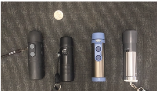
Fig. 9.1 Electrolarynges with quarter for scale. From left: (a) NuVois III Digital™; (b) TruTone™; (c) Servox® Inton; (d) Romet® R210. (Photo by K.F. Nagle)
