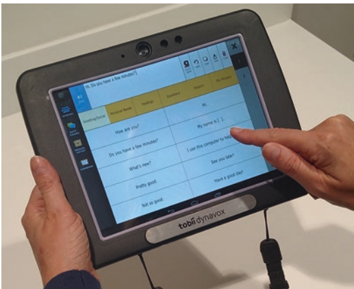
Fig. 15.2 An example of a dedicated speech-generating device with synthesized speech. (Tobii Dynavox T-10, Tobii Dynavox, Pittsburgh, PA)
