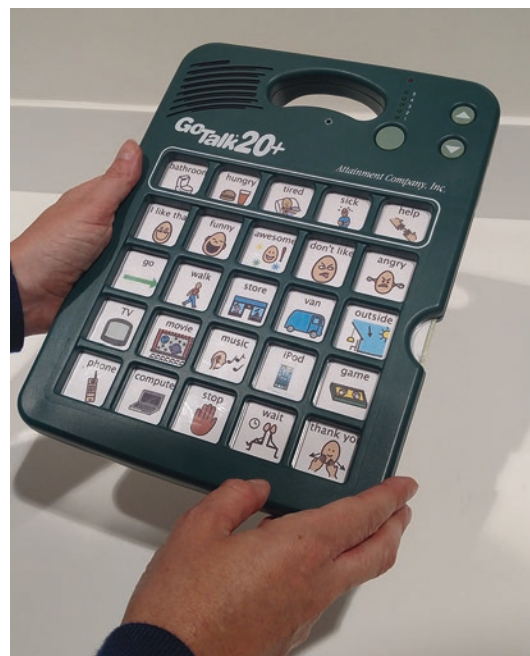
Fig. 15.1 An example of a dedicated speech-generating device with digitized speech. (GoTalk 20+, Attainment Company, Verona, WI)
