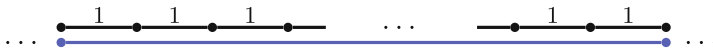
Fig. 1. Greedy online algorithm for DPA which satisfies the first request (lowest one) and has to reject all subsequent small requests of length 1.
