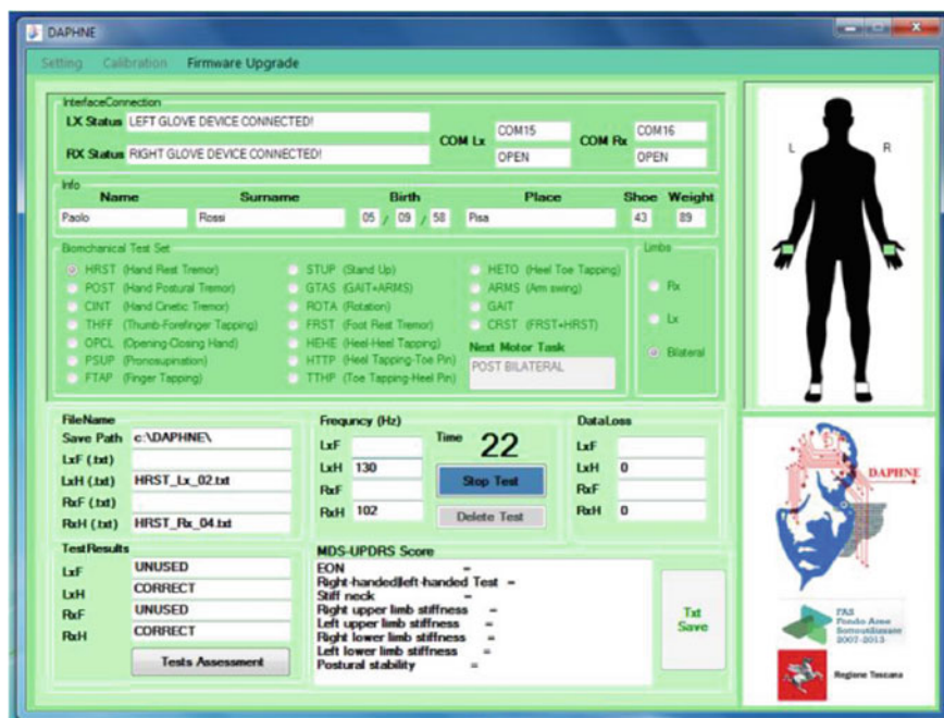
Fig. 3 DAPHNE clinical interface. Such interface is composed by: an upper part in which is possible to control linked sensorized wearable devices status (Interface Connection); an Info section in which patient personal data can be inserted; a Biomechanical Test Set acting as control panel to choose which task the patient is asked to perform; a lower section in which feedbacks about the test results and the saving path can be controlled; a section in which feedback about the frequency at which devices are acquiring can be checked; a task timer; a Data Loss section sending an alert in case the test is failing; a MDS-UPDRS section in which the assigned score is shown
