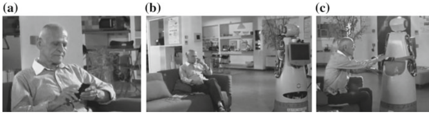
Fig. 2 Mobility application a the elderly user calls ASTRO robot because he needs to go to another room, b ASTRO robot arrives, c the user uses ASTRO handle and together go to the desired room
