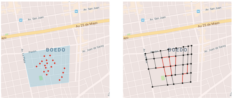
Fig. 1. (a) A possible set of customers, marked as red dots, on a small part of Boedo neighborhood in Buenos Aires. The light blue area is an arbitrary boundary for the truck. (b) A STAR instance that models the problem. Red edges are blocks that contain customers. (Color figure online)
