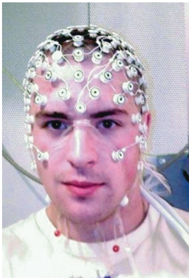
Fig. 7.2 An example of a head cap for the EEG high-density recording (photograph of public domain on web)
