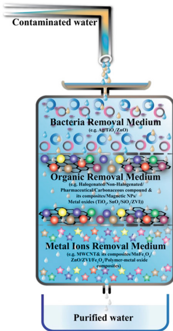
Fig. 1.6 Nanomaterial-packed layer for purification of water contaminants
