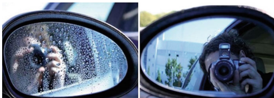
Fig. 11.13 Photographs of antifogging automotive side view mirror: uncoated (left) and coated (right) with \text{TiO}_2 . (Reprinted from Zhang et al. (2012) with permission of the Royal Society of Chemistry)
