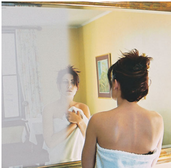
Fig. 11.14 Photograph of super-hydrophilic-coated antifogging mirrors. (Reprinted from Gould (2003) with permission from Elsevier)
