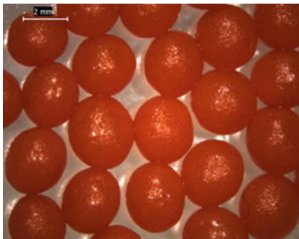
Fig. 9.15 Optical microscopic picture of Fe-Zr entrapped calcium alginate. (Reprinted from Swain et al. 2013)
