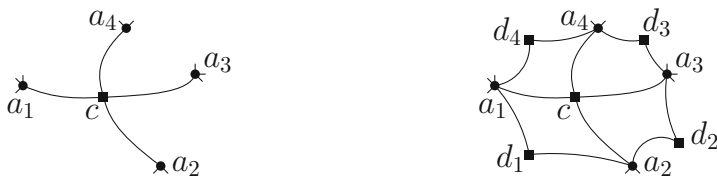
(a) Planarized crossing where the crossing point became a crossing vertex c . (b) Enclosing the crossing vertex c by a subdivided kite.
