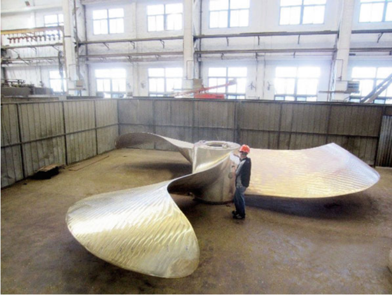
Fig. 2.2 Three-bladed Kappel propeller. (Courtesy MAN)
