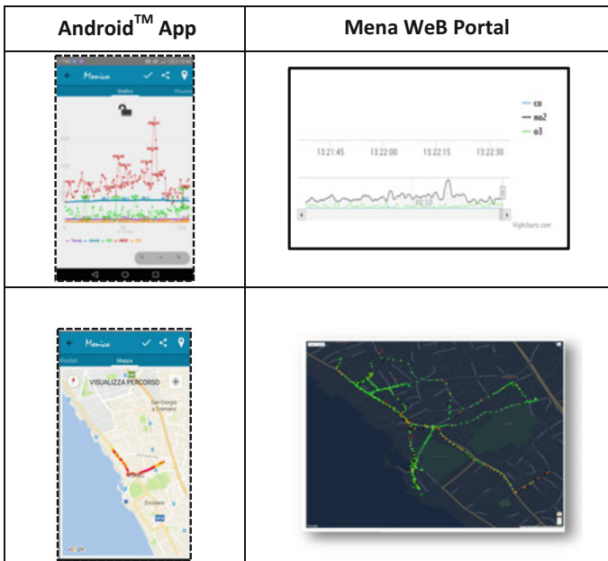
Fig. 5 On the top, trend of pollutants during an user session on app (left) and web interface (right). On the bottom, colored 2D route map on smartphone app (left) and web interface (right)
