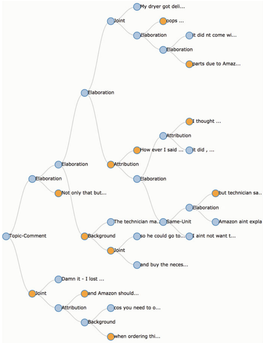
Fig. 13.24 Default discourse tree obtained for noisy text directly, without using NCDT algorithm: certain relations such as Contrast and Attribution are lost (compared to NCDT above)
