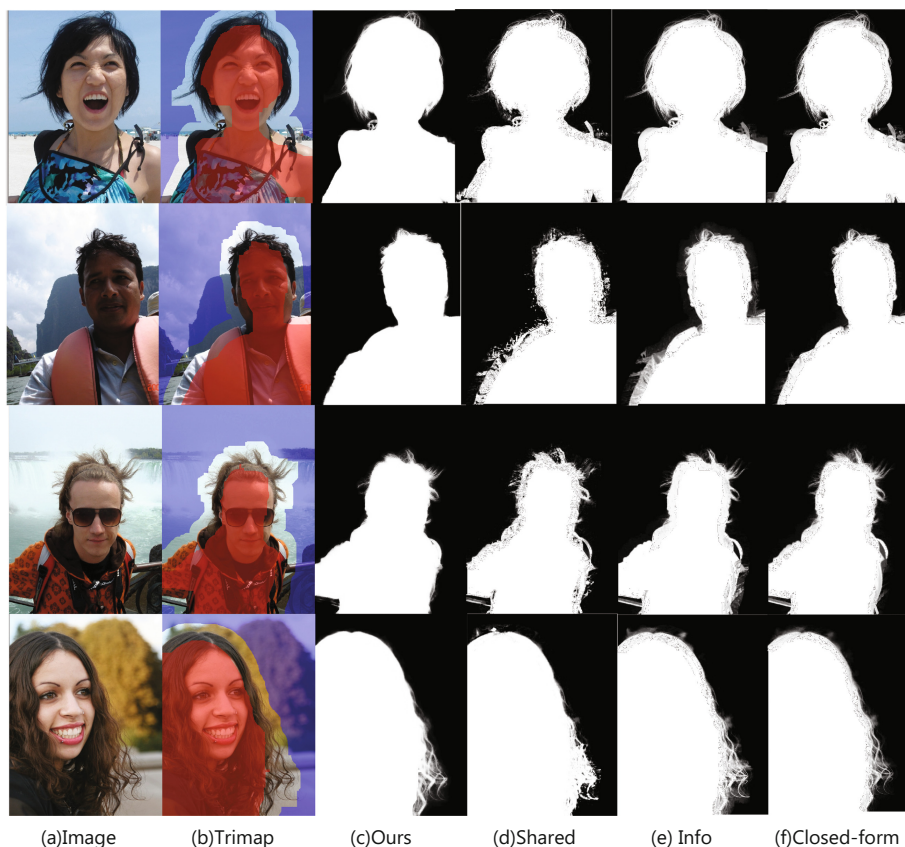
Fig. 5. Visual comparisons on 2k portrait matting dataset. (a) Image (b) Trimap (c) Ours (d) Shared-Matting [8] (e) Information-flow [1] (e) Closed-form [11]
