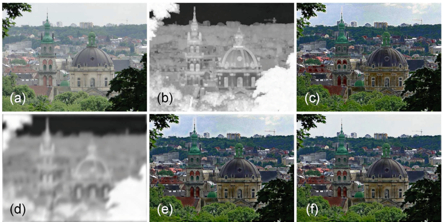
Fig. 1. Framework of our proposed dehazing method: (a) input hazy image, (b) coarse transmission map t_0 using DCP, (c) dehazing result with (b), (d) refined transmission map t using our two-phase estimation method, (e) initial dehazing result with (d), (f) final dehazing result with a tolerance mechanism implemented for (e).
