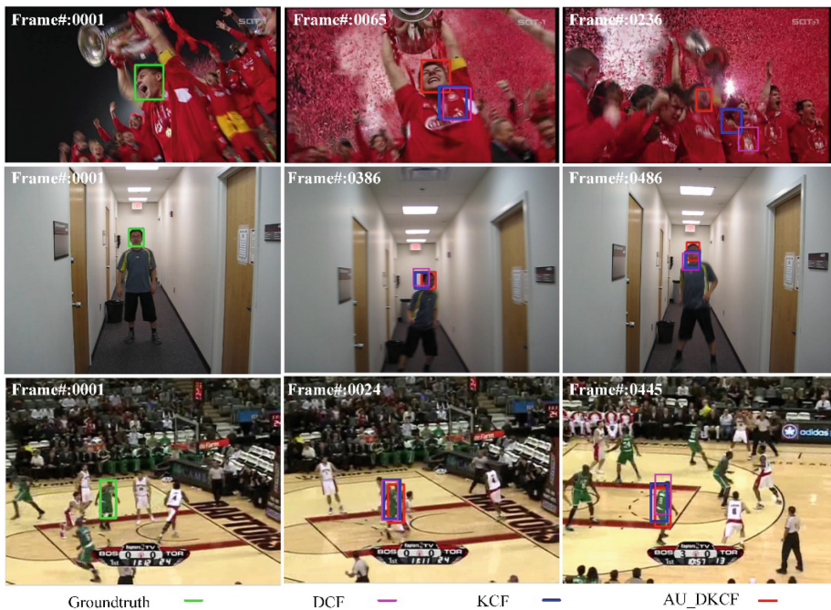
Fig. 5. Tracking results of two baseline CF trackers compared to proposed AU_DKCF. Videos are (from top to bottom): Soccer, Boy and Basketball
