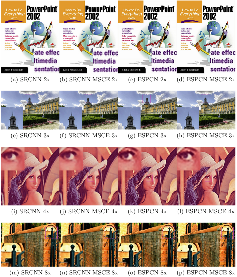
Fig. 5. Comparison of the results obtained on down-sampled (by bicubic interpolation without blurring) images on different upscaling factors. (a), (b), (c) and (d) have been down-sampled by a factor of 2 and reconstructed. (e), (f), (g) and (h) have been down-sampled by a factor of 3 and reconstructed. (i), (j), (k) and (l) have been down-sampled by a factor of 4 and reconstructed. (m), (n), (o) and (p) have been down-sampled by a factor of 8 and reconstructed.
