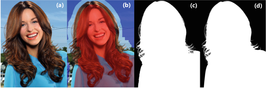
Fig. 1. (a) Image from our Synthetic dataset( 1280 \times 960 pixels). (b) Trimap. Red color stands for definite foreground and blue color stands for definite background. The rest of the region stands for unknown. (c) Result of Our SDPNet. The running time is 40ms on GPU. (d) Our labeled groundtruth.
