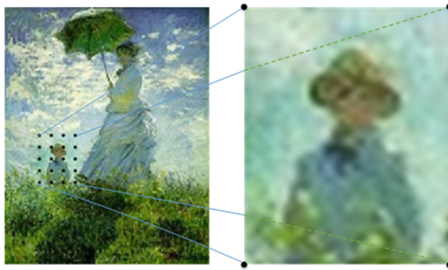
Fig. 1. An illustration of zoom-in transformation achieved by sampling. Blue lines indicate mappings. Black points represent sampling grid. (Color figure online)
