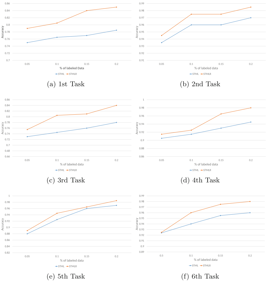
Fig. 3. Performance on the handwritten letter classification with one target task and other tasks as source tasks in STML and STMLR
