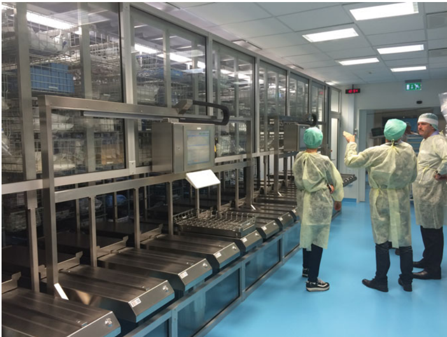
Fig. 1 AS/RS system in Denmark Health CSSD
