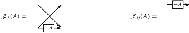
Fig. 6 Graph representing the active part of the block elementary Fiedler factor \mathcal{F}_i(A) , for i > 0 and of \mathcal{F}_0(A)
