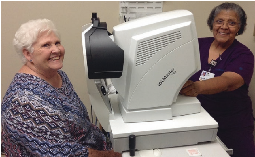
Fig. 1 New technology allows more accurate calculation of intraocular lens power, decreasing the patient's postoperative spectacle dependence. (Optical biometry, in this case the IOLMaster)
