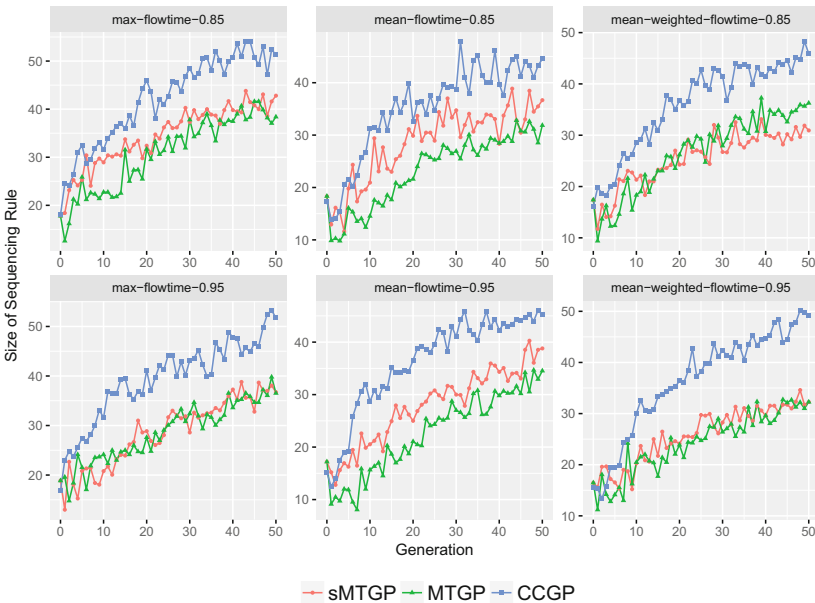
Fig. 4. The convergence curves of the average best sequencing rule size (30 runs) obtained by sMTGP, MTGP and CCGP at each generation.
