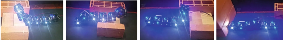
Fig. 5. Frames of the EMeRGE robot evading an obstacle in the form of a ladder.
