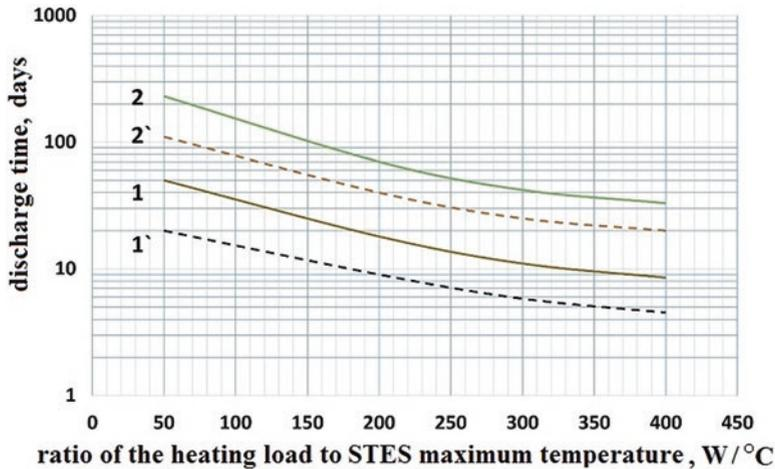
**Fig. 9.4** STES discharge time in the modes of complete discharge (1, 2) and discharge to 35 °C (1', 2') with the storage capacity of 100 and 500 m<sup>3</sup>
