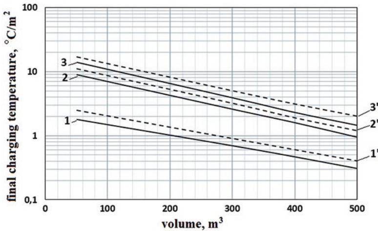
Fig. 9.3 The final temperature of STES charging per square meter of solar collector area (in Yekaterinburg): 1, 2, 3 and 1', 2', 3' are the charging time during 1, 3, and 6 summer months at  $T_k$  of 75 °C and 50 °C, respectively
