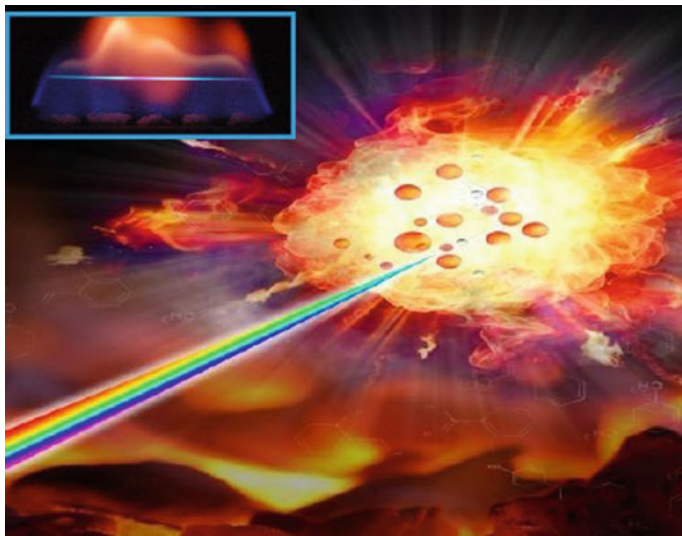
Fig. 10.1 Concept of combustion diagnostic based on femtosecond laser filament-induced nonlinear spectroscopy. The self-channeling laser-induced intense laser intensity induces the ionization and excitation of combustion intermediates which emit characteristic optical radiations. Inset shows a photo of a laser-induced filament in a combustion flame in air with a methanol fuel gas produced by the irradiation of near-IR femtosecond laser pulses (800 nm, 40 fs, and 5.5 mJ/pulse)
