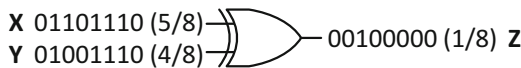
Fig. 4 XOR gate with maximal positively correlated inputs which implements the absolute-difference subtraction function |X - Y| [2]
