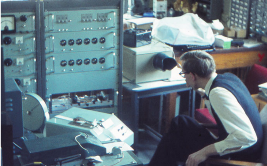
Fig. 5 Brian Gaines working with the analog computer and stereoscopic oscilloscope that he built, Department of Experimental Psychology, Cambridge, 1964
