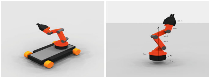
Fig. 6 Configuration of a KUKA youBot with an omnidirectional platform and a five link robotic arm
