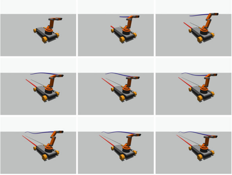
Fig. 11 Snapshots of the motion of the mobile robot (Example 3.3): Tracking of a prescribed path for the end effector from t = 0 (top left) to t = 2\pi (bottom right). Please note that the wheels are omnidirectional (although they appear as standard wheels in the graphics)
