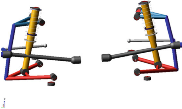
Fig. 3 Multibody system model of an axle with double wishbone suspensions, screenshot from the software tool ADAMS
