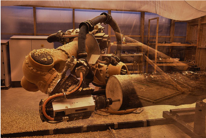
Fig. 5 AA, Woodchip Barn: complex joints made by robotic milling process. © Genny Spyridonos
