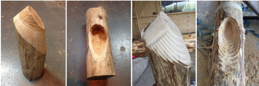
Fig. 6 AA, Woodchip Barn: complex joints made by milling process informed by data-driven design. © Swetha Vegesana
