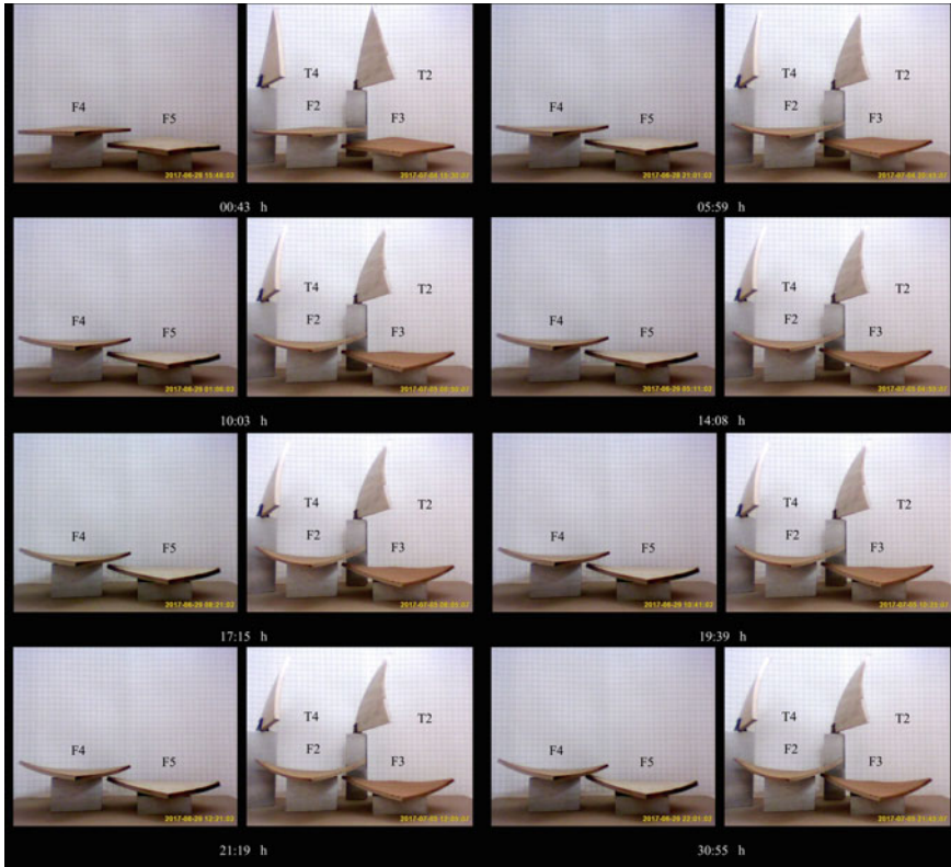
Fig. 6 Modelling as result of observation of phenomena: curvature in function of the humidity in climatic chamber tests
