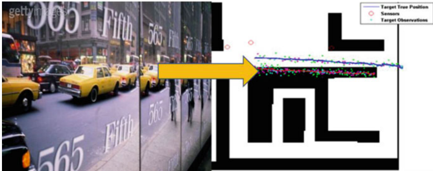
Fig. 11.4 Tracking of city traffic by video sensors. False detections are generated by a reflective surface and false tracks could be generated
